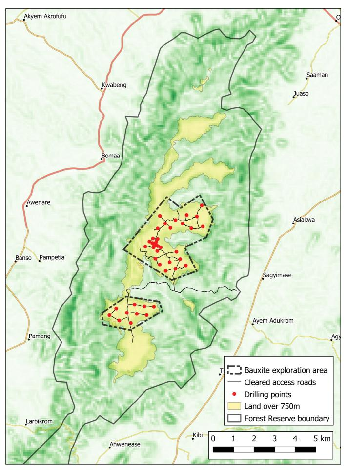
Bauxite exploration area based on map provided by GIADEC.750 m contour based on Shuttle Radar data. Green shading = steepness of slope. Drainage network from TEEB dataset with some local adjustments. UTM 30N. A Rocha 8 January 2020.
