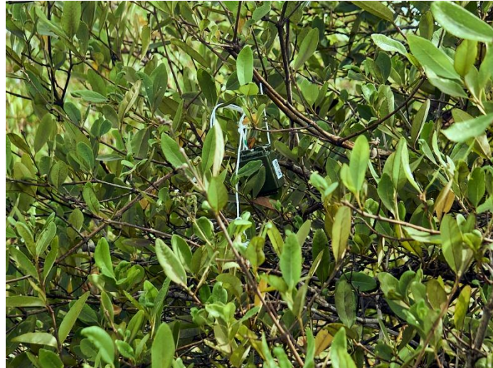
Figure 3: Sound recorder Song Meter Micro 2 deployed in Keta Lagoon Complex Ramsar Site in February 2025.
